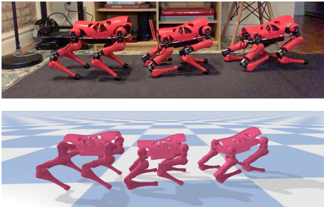
Fig. 6. Transfer of our forward gait policy with a gait trained on an automatically tuned simulator. The bottom figure pictures the gait on our baseline hand-tuned simulator and the top figure shows the real robot successfully moving forward using a policy trained using our approach.
